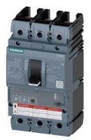
Circuit breaker 3VA6 UL frame 250 breaking capacity class H 65kA @ 480V 3-pole, Line protection ETU320, LI, In=100A overload protection, 100% rated Ir=40A...100A Short-circuit protection Ii=1.5...12 x In without connection
