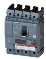
Circuit breaker 3VA6 UL frame 250 breaking capacity class M 35kA @ 480V 4pole, Line protection ETU856, LSI, In=100A overload protection, 100% rated Ir=40A...100A Short-circuit protection Isd=0.6..10x In, Ii=1.5..12x In N conductor protection adjustable (OFF, up to 160%) Ground-fault alarm message via EFB300 or COM without connection
