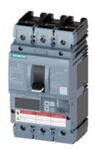
Circuit breaker 3VA6 UL frame 250 breaking capacity class M 35kA @ 480 V 3-pole, Line protection ETU856, LSI, In=100A overload protection, 100% rated Ir=40A ...100A Short-circuit protection Isd=0.6..10x In, Ii=1.5..12x In N conductor protection optionally with external CT; up to 160% Ground-fault alarm message via EFB300 or COM cable connection on both sides
