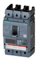
Circuit breaker 3VA6 UL frame 250 breaking capacity class M 35kA @ 480V 3-pole, Line protection ETU856, LSI, In=100A overload protection, 100% rated Ir=40A...100A Short-circuit protection Isd=0.6..10x In, Ii=1.5..12x In N conductor protection optionally with external CT, up to 160% Ground-fault alarm message via EFB300 or COM without connection
