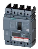
Circuit breaker 3VA6 UL frame 250 breaking capacity class M 35kA @ 480V 4-pole, Line protection ETU860, LSIG, In=100A overload protection, 100% rated Ir=40A...100A Short-circuit protection Isd=0.6..10x In, Ii=1.5..12x In N conductor protection adjustable (OFF, up to 160%) Ground-fault protection Ig=0.2...1 x In=tg=0.05-0.8s without connection
