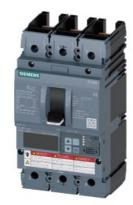
Circuit breaker 3VA6 UL frame 250 breaking capacity class M 35kA @ 480V 3-pole, Line protection ETU860, LSIG, In=100A overload protection, 100% rated Ir=40A...100A Short-circuit protection Isd=0.6..10x In, Ii=1.5..12x In N conductor protection optionally with external CT, up to 160% Ground-fault protection Ig=0.2...1 x In, tg=0.05-0.8s without connection
