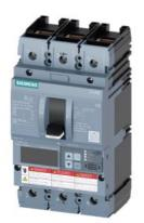
circuit breaker 3VA6 UL frame 250 breaking capacity class M 35kA @ 480 V 3-pole, line protection ETU850, LSI, In=100A overload protection Ir=40A ...100A short-circuit protection Isd=0.6..10x In, Ii=1.5..12x In N conductor protection opt. w. ext. CT; up to 160% cable connection on both sides
