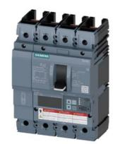
Circuit breaker 3VA6 UL frame 250 breaking capacity class M 35kA @ 480V 4-pole, Line protection ETU830, LIG, In=100A overload protection, 100% rated Ir=40A...100A Short-circuit protection Ii=1.5...12 x In Ground-fault protection Ig=0.2...1 x In, tg=0.05-0.8s without connection
