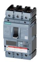
Circuit breaker 3VA6 UL frame 250 breaking capacity class M 35kA @ 480 V 3-pole, Line protection ETU830, LIG, In=100A overload protection, 100% rated Ir=40A ...100A Short-circuit protection Ii=1.5...12 x In Ground-fault protection Ig=0.2... 1 x In, tg=0.05-0.8s cable connection on both sides
