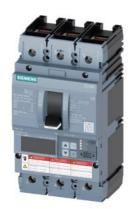
circuit breaker 3VA6 UL frame 250 breaking capacity class M 35kA @ 480 V 3-pole, line protection ETU830, LIG, ln=100A overload protection lr=40A ...100A short-circuit protection li=1.5...12 x ln ground-fault protection lg=0.2... 1 x ln, tg=0.05-0.8s cable connection on both sides
