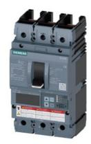
Circuit breaker 3VA6 UL frame 250 breaking capacity class M 35kA @ 480V 3-pole, Line protection ETU830, LIG, In=100A overload protection, 100% rated Ir=40A...100A Short-circuit protection Ii=1.5...12 x In Ground-fault protection Ig=0.2...1 x In, tg=0.05-0.8s without connection
