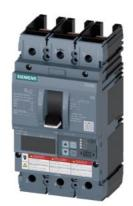
circuit breaker 3VA6 UL frame 250 breaking capacity class M 35kA @ 480V 3-pole, line protection ETU830, LIG, In=100A overload protection Ir=40A...100A short-circuit protection Ii=1.5...12 x In ground-fault protection Ig=0.2...1 x In, tg=0.05-0.8s without connection
