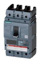
Circuit breaker 3VA6 UL frame 250 breaking capacity class M 35kA @ 480V 3-pole, Line protection ETU820, LI, In=100A overload protection, 100% rated Ir=40A...100A Short-circuit protection Ii=1.5...12 x In without connection
