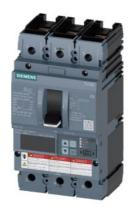
Circuit breaker 3VA6 UL frame 250 breaking capacity class M 35kA @ 480 V 3-pole, Line protection ETU556, LSI, In=100A overload protection, 100% rated Ir=40A ...100A Short-circuit protection Isd=0.6..10x In, Ii=1.5..12x In N conductor protection optionally with external CT; up to 160% Ground-fault alarm message via EFB300 or COM nut keeper kit on both sides
