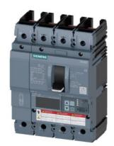
Circuit breaker 3VA6 UL frame 250 breaking capacity class M 35kA @ 480V 4-pole, Line protection ETU560, LSIG, In=100A overload protection, 100% rated Ir=40A...100A Short-circuit protection Isd=0.6..10x In, Ii=1.5..12x In N conductor protection adjustable (OFF, up to 160%) Ground-fault protection Ig=0.2...1 x In=tg=0.05-0.8s without connection
