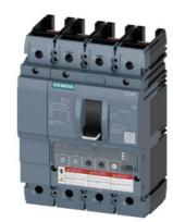
circuit breaker 3VA6 UL frame 250 breaking capacity class M 35kA @ 480V 4-pole, line protection ETU330, LIG, In=100A overload protection Ir=40A...100A short-circuit protection Ii=1.5...12 x In N conductor protection adjustable (OFF, 50%, 100%) ground-fault protection Ig=0.2...1 x In= tg=0.1/0.3s without connection
