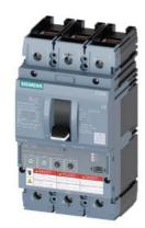
Circuit breaker 3VA6 UL frame 250 breaking capacity class M 35kA @ 480 V 3pole, Line protection ETU330, LIG, In=100A overload protection, 100% rated Ir=40A ...100A Short-circuit protection Ii=1.5...12 x In Ground-fault protection Ig=0.2... 1 x In, tg=0.1/0.3s cable connection on both sides
