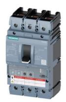
circuit breaker 3VA6 UL frame 250 breaking capacity class M 35kA @ 480 V 3-pole, line protection ETU330, LIG, ln=100A overload protection lr=40A ...100A short-circuit protection li=1.5...12 x ln ground-fault protection lg=0.2... 1 x ln, tg=0.1/0.3s cable connection on both sides
