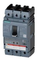
circuit breaker 3VA6 UL frame 250 breaking capacity class M 35kA @ 480 V 3-pole, line protection ETU330, LIG, ln=100A overload protection lr=40A ...100A short-circuit protection li=1.5...12 x ln ground-fault protection lg=0.2... 1 x ln, tg=0.1/0.3s nut keeper kit on both sides
