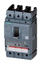
Circuit breaker 3VA6 UL frame 250 breaking capacity class M 35kA @ 480V 3-pole, Line protection ETU330, LIG, In=100A overload protection, 100% rated Ir=40A...100A Short-circuit protection Ii=1.5...12 x In Ground-fault protection Ig=0.2...1 x In, tg=0.1/0.3s without connection
