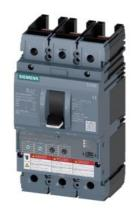
circuit breaker 3VA6 UL frame 250 breaking capacity class M 35kA @ 480V 3-pole, line protection ETU330, LIG, In=100A overload protection Ir=40A...100A short-circuit protection Ii=1.5...12 x In ground-fault protection Ig=0.2...1 x In, tg=0.1/0.3s without connection
