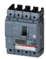
circuit breaker 3VA6 UL frame 150 breaking capacity class C 100kA @ 480V 4pole, line protection ETU856, LSI, In=40A overload protection Ir=16A...40A shortcircuit protection Isd=0.6..10x In, Ii=1.5..12x In N conductor protection adjustable (OFF, up to 160%) ground-fault alarm message via EFB300 or COM without connection
