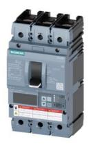
Circuit breaker 3VA6 UL Frame 150 breaking capacity class C 100kA @ 480 V 3-pole, Line protection ETU856, LSI, In=40A overload protection, 100% rated Ir=16A ...40A Short-circuit protection Isd=0.6...10x In, Ii=1.5..12x In N conductor protection optionally with external CT; up to 160% Ground-fault alarm message via EFB300 or COM cable connection on both sides
