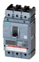
circuit breaker 3VA6 UL frame 150 breaking capacity class C 100kA @ 480 V 3-pole, line protection ETU856, LSI, In=40A overload protection Ir=16A ...40A short-circuit protection Isd=0.6..10x In, Ii=1.5..12x In N conductor protection opt. w. ext. CT; up to 160% ground-fault alarm message via EFB300 or COM cable connection on both sides
