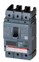
Circuit breaker 3VA6 UL Frame 150 breaking capacity class C 100kA @ 480V 3-pole, Line protection ETU856, LSI, In=40A overload protection, 100% rated Ir=16A...40A Short-circuit protection Isd=0.6..10x In, Ii=1.5..12x In N conductor protection optionally with external CT, up to 160% Ground-fault alarm message via EFB300 or COM without connection
