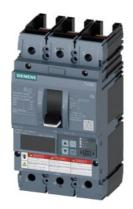
circuit breaker 3VA6 UL frame 150 breaking capacity class C 100kA @ 480V 3-pole, line protection ETU856, LSI, In=40A overload protection Ir=16A...40A short-circuit protection Isd=0.6..10x In, Ii=1.5...12x In N conductor protection optionally with external current transformer, up to 160% ground-fault alarm message via EFB300 or COM without connection
