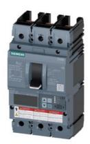
Circuit breaker 3VA6 UL Frame 150 breaking capacity class C 100kA @ 480V 3-pole, Line protection ETU850, LSI, In=40A overload protection, 100% rated Ir=16A...40A Short-circuit protection Isd=0.6..10x In, Ii=1.5..12x In N conductor protection optionally with external CT, up to 160% without connection
