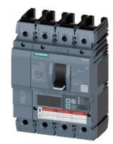
Circuit breaker 3VA6 UL Frame 150 breaking capacity class C 100kA @ 480V 4-pole, Line protection ETU830, LIG, In=40A overload protection, 100% rated Ir=16A...40A Short-circuit protection Ii=1.5...12 x In Ground-fault protection Ig=0.375...1 x In, tg=0.05-0.8s without connection
