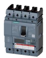
circuit breaker 3VA6 UL frame 150 breaking capacity class C 100kA @ 480V 4-pole, line protection ETU830, LIG, In=40A overload protection Ir=16A...40A short-circuit protection Ii=1.5...12 x In ground-fault protection Ig=0.375...1 x In, tg=0.05-0.8s without connection
