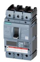
Circuit breaker 3VA6 UL Frame 150 breaking capacity class C 100kA @ 480 V 3-pole, Line protection ETU830, LIG, In=40A overload protection, 100% rated Ir=16A ...40A Short-circuit protection Ii=1.5...12 x In Ground-fault protection Ig=0.375...1x In, tg=0.05-0.8s cable connection on both sides
