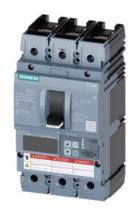
circuit breaker 3VA6 UL frame 150 breaking capacity class C 100kA @ 480 V 3pole, line protection ETU830, LIG, In=40A overload protection Ir=16A ...40A shortcircuit protection Ii=1.5...12 x In ground-fault protection Ig=0.375...1x In, tg=0.05-0.8s cable connection on both sides
