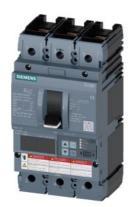
Circuit breaker 3VA6 UL Frame 150 breaking capacity class C 100kA @ 480 V 3-pole, Line protection ETU830, LIG, In=40A overload protection, 100% rated Ir=16A ...40A Short-circuit protection Ii=1.5...12 x In Ground-fault protection Ig=0.375...1x In, tg=0.05-0.8s nut keeper kit on both sides
