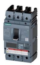
Circuit breaker 3VA6 UL Frame 150 breaking capacity class C 100kA @ 480V 3-pole, Line protection ETU830, LIG, In=40A overload protection, 100% rated Ir=16A...40A Short-circuit protection Ii=1.5...12 x In Ground-fault protection Ig=0.375...1 x In, tg=0.05-0.8s without connection
