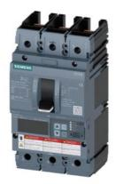
circuit breaker 3VA6 UL frame 150 breaking capacity class C 100kA @ 480V 3-pole, line protection ETU820, LI, In=40A overload protection Ir=16A...40A short-circuit protection Ii=1.5...12 x In without connection
