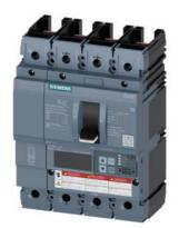
circuit breaker 3VA6 UL frame 150 breaking capacity class C 100kA @ 480V 4-pole, line protection ETU560, LSIG, In=40A overload protection Ir=16A...40A short-circuit protection Isd=0.6..10x In, Ii=1.5..12x In N conductor protection adjustable (OFF, up to 160%) ground-fault protection Ig=0.375...1 x In= tg=0.05-0.8s without connection
