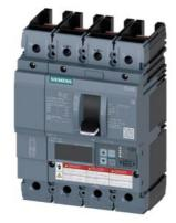
circuit breaker 3VA6 UL frame 150 breaking capacity class C 100kA @ 480V 4-pole, line protection ETU550, LSI, In=40A overload protection Ir=16A...40A short-circuit protection Isd=0.6..10x In, Ii=1.5..12x In N conductor protection adjustable (OFF, up to 160%) without connection
