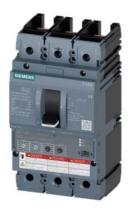
Circuit breaker 3VA6 UL Frame 150 breaking capacity class C 100kA @ 480V 3-pole, Line protection ETU350, LSI, In=40A overload protection, 100% rated Ir=16A...40A Short-circuit protection Isd=1.5...10 x Ir, Ii=12 x In without connection
