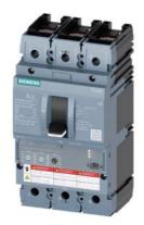
Circuit breaker 3VA6 UL Frame 150 breaking capacity class C 100kA @ 480 V 3-pole, Line protection ETU320, LI, In=40A overload protection, 100% rated Ir=16A ...40A Short-circuit protection li=1.5...12 x In cable connection on both sides
