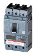
Circuit breaker 3VA6 UL Frame 150 breaking capacity class H 65kA @ 480 V 3pole, Line protection ETU856, LSI, In=40A overload protection, 100% rated Ir=16A ...40A Short-circuit protection Isd=0.6..10x In, Ii=1.5..12x In N conductor protection optionally with external CT; up to 160% Ground-fault alarm message via EFB300 or COM cable connection on both sides
