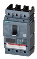
Circuit breaker 3VA6 UL Frame 150 breaking capacity class H 65kA @ 480V 3-pole, Line protection ETU856, LSI, In=40A overload protection, 100% rated Ir=16A...40A Short-circuit protection Isd=0.6..10x In, Ii=1.5..12x In N conductor protection optionally with external CT, up to 160% Ground-fault alarm message via EFB300 or COM without connection
