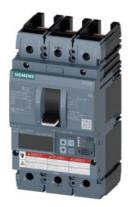
circuit breaker 3VA6 UL frame 150 breaking capacity class H 65kA @ 480V 3-pole, line protection ETU856, LSI, In=40A overload protection Ir=16A...40A short-circuit protection Isd=0.6..10x In, Ii=1.5..12x In N conductor protection optionally with external current transformer, up to 160% ground-fault alarm message via EFB300 or COM without connection
