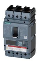
circuit breaker 3VA6 UL frame 150 breaking capacity class H 65kA @ 480 V 3-pole, line protection ETU860, LSIG, In=40A overload protection Ir=16A ...40A short-circuit protection Isd=0.6..10x In, Ii=1.5..12x In N conductor protection opt. w. ext. CT; up to 160% ground-fault protection Ig=0.375...1x In, tg=0.05-0.8s nut keeper kit on both sides
