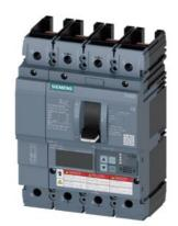
Circuit breaker 3VA6 UL Frame 150 breaking capacity class H 65kA @ 480V 4-pole, Line protection ETU830, LIG, In=40A overload protection, 100% rated Ir=16A...40A Short-circuit protection li=1.5...12 x In Ground-fault protection lg=0.375...1 x In, tg=0.05-0.8s without connection
