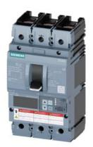
circuit breaker 3VA6 UL frame 150 breaking capacity class H 65kA @ 480 V 3-pole, line protection ETU830, LIG, ln=40A overload protection lr=16A ...40A short-circuit protection li=1.5...12 x ln ground-fault protection lg=0.375...1x ln, tg=0.05-0.8s cable connection on both sides
