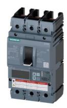
circuit breaker 3VA6 UL frame 150 breaking capacity class H 65kA @ 480V 3-pole, line protection ETU830, LIG, In=40A overload protection Ir=16A...40A short-circuit protection Ii=1.5...12 x In ground-fault protection Ig=0.375...1 x In, tg=0.05-0.8s without connection
