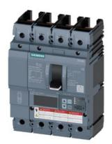
Circuit breaker 3VA6 UL Frame 150 breaking capacity class H 65kA @ 480V 4-pole, Line protection ETU556, LSI, In=40A overload protection, 100% rated Ir=16A...40A Short-circuit protection Isd=0.6..10x In, Ii=1.5..12x In N conductor protection adjustable (OFF, up to 160%) Ground-fault alarm message via EFB300 or COM without connection
