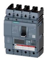
circuit breaker 3VA6 UL frame 150 breaking capacity class H 65kA @ 480V 4-pole, line protection ETU556, LSI, In=40A overload protection Ir=16A...40A short-circuit protection Isd=0.6..10x In, Ii=1.5..12x In N conductor protection adjustable (OFF, up to 160%) ground-fault alarm message via EFB300 or COM without connection
