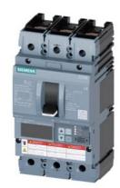
Circuit breaker 3VA6 UL Frame 150 breaking capacity class H 65kA @ 480 V 3pole, Line protection ETU556, LSI, In=40A overload protection, 100% rated Ir=16A ...40A Short-circuit protection Isd=0.6..10x In, Ii=1.5..12x In N conductor protection optionally with external CT; up to 160% Ground-fault alarm message via EFB300 or COM cable connection on both sides
