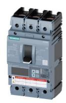
circuit breaker 3VA6 UL frame 150 breaking capacity class H 65kA @ 480 V 3pole, line protection ETU556, LSI, In=40A overload protection Ir=16A ...40A shortcircuit protection Isd=0.6..10x In, Ii=1.5..12x In N conductor protection opt. w. ext. CT; up to 160% ground-fault alarm message via EFB300 or COM cable connection on both sides
