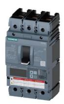
Circuit breaker 3VA6 UL Frame 150 breaking capacity class H 65kA @ 480 V 3-pole, Line protection ETU556, LSI, In=40A overload protection, 100% rated Ir=16A ...40A Short-circuit protection Isd=0.6..10x In, Ii=1.5..12x In N conductor protection optionally with external CT; up to 160% Ground-fault alarm message via EFB300 or COM nut keeper kit on both sides
